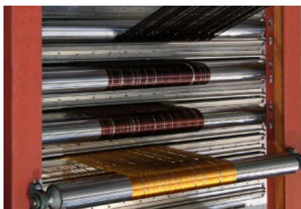
PAN fiber going through oxidation oven
